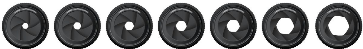
*Example of an aperture in various sizes from smallest to largest
